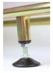
The forward-most crossbar uses a pair of adjustable rubber feet and has an extra M6 Nyloc nut and bolt at the end to prevent it from turning. Drop this into place but again, don't tighten everything fully yet.
