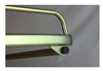
...and fit the roller at the back as you install the other side. The bearings are made from self-lubricating Nylotron (graphite impregnated nylon) and need no additional lubrication.
