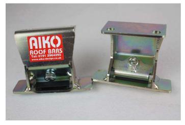
You can probably see how the brackets fit- the lip on the bottom slots under the lip in the van roof, and the little rubber-edged clamp does up with an M8 bolt and spring washer to secure it all in place.
